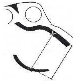
Figure 6-18. Cat head diameter measurement sketch
