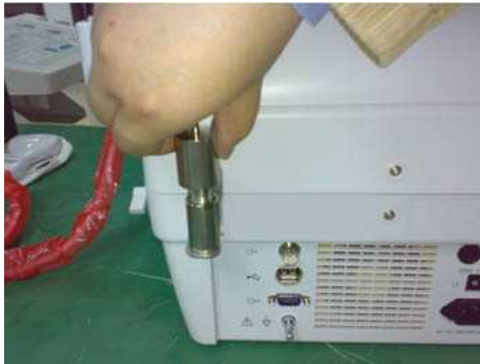
Figure 4-4 Installing the probe hook step 2
