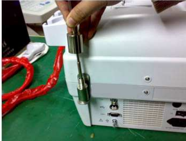
Figure 4-3 Installing the probe hook step 1
