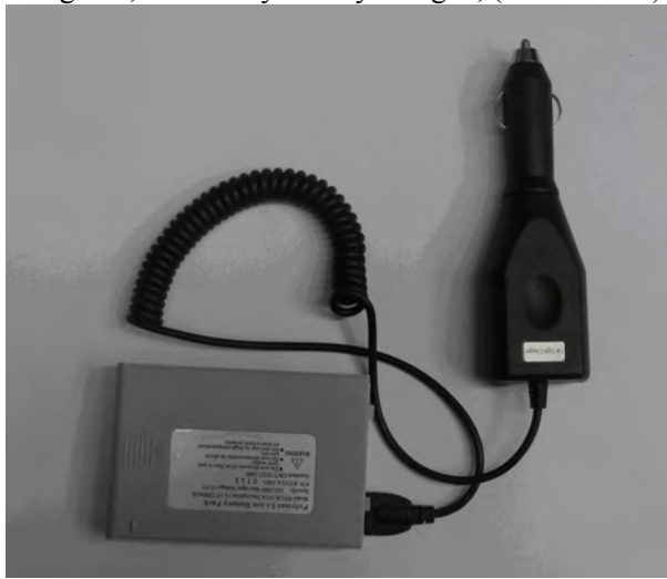
Picture 2-5. AV-2100V charging through auto-charger
